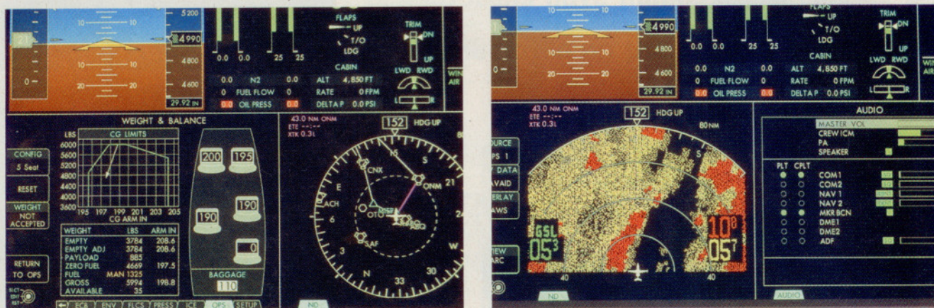
Garmin 400s (top, just below the PFDs) provide FMS-like capability in the Avio NG 1.5 panel. Graphical weight and balance on the MFD’s Ops page (above, left) eases preflight. It can also show navigation mapping. TAWS information can also be overlaid (above, right).
