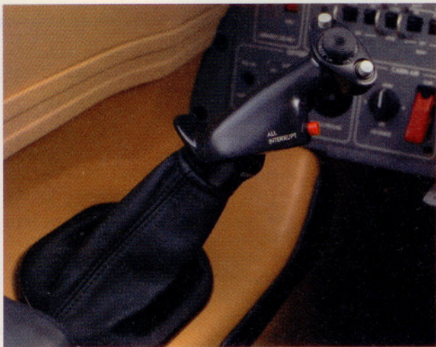
Thanks to FADEC, engine start is a simple turn of a knob on the overhead (above, left). A deft touch is necessary on the thrust levers to eke it out of takeoff thrust to max continuous (above). Landing flap speed was recently increased from 120 to 140 knots. Part of the training includes mastering the sidestick (left), which is festooned with buttons for autopilot disconnect, gear horn silence, trim interrupt, transponder ID, push-to-talk, and a hat switch for elevator and aileron trim.
