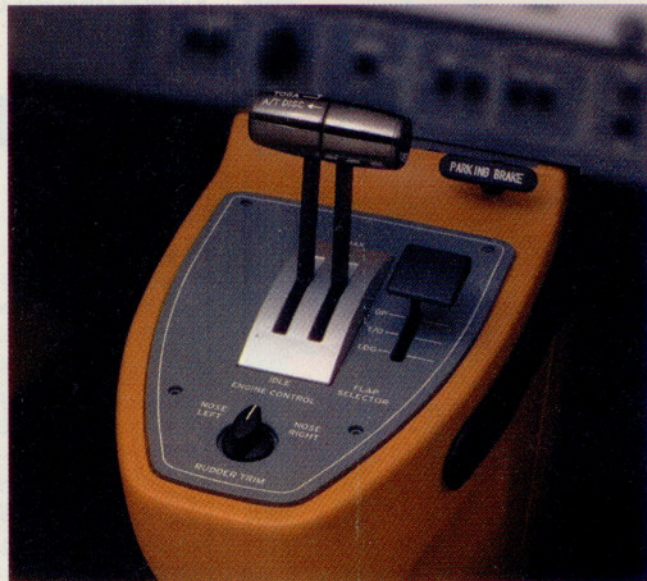
Thanks to FADEC, engine start is a simple turn of a knob on the overhead (above, left). A deft touch is necessary on the thrust levers to eke it out of takeoff thrust to max continuous (above). Landing flap speed was recently increased from 120 to 140 knots. Part of the training includes mastering the sidestick (left), which is festooned with buttons for autopilot disconnect, gear horn silence, trim interrupt, transponder ID, push-to-talk, and a hat switch for elevator and aileron trim.
