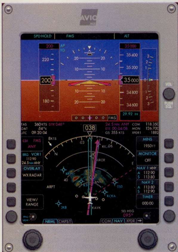
The pilot can choose to overlay weather radar and nav aids on the HSI (above).
