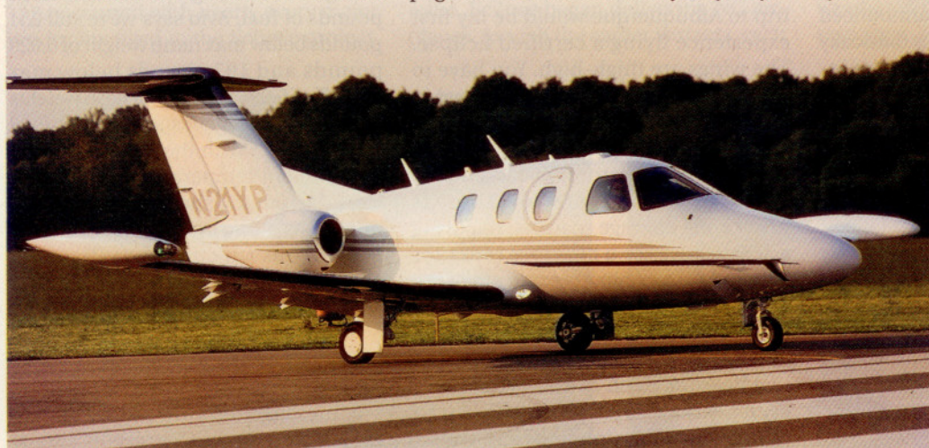
Eclipse uses long-life, low-power LEDs for navigation and many other lights throughout the airplane. The air conditioning inlet/exhaust doors are open here (bottom of the nose).
